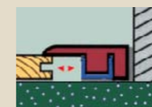
End profile For proper borders of different floor surfaces in front of adjacent sills, tiles, etc.
