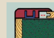
Staircase profile For staircase nosing cover at the edge between the riser and step.
